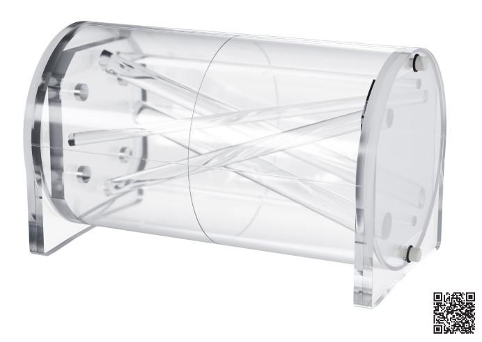
The Phantom designed for a simple and cost effective **verification of image alignment and distortion in hybrid scanning systems like PET/CT or NM/CT**. It consists of a cylinder that can be filled with a variety of fluids. Several non-parallel rods of varying diameter and at certain angles in relation to the phantom's axes run the entire length of the cylinder. Images produced with different modalities allow quick and **simple identification of misalignments on fused studies**.
